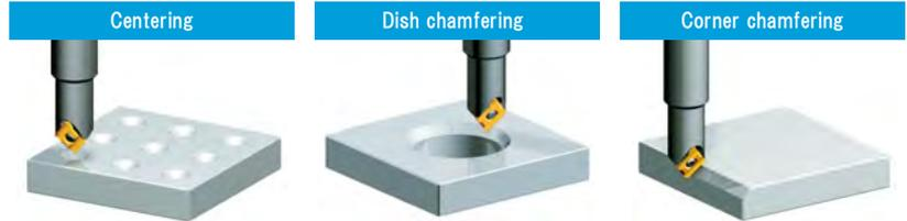
※ This tool cannot be used with drilling machines
